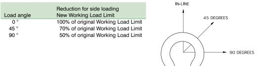
In-line loading is considered to be a load perpendicular to the pin and in the plane of the bow. Load angles in the table are the deviating angles from the in line loads.
