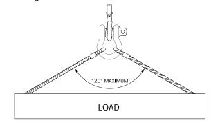
When a shackle is used to connect two slings to the hook of a lifting device, a bow type shackle must be assembled with the slings in the shackle body and the hook engaged with the shackle pin. The angle between the slings should not exceed 120°. If symmetrically loaded the shackle may be used to the full WLL.
